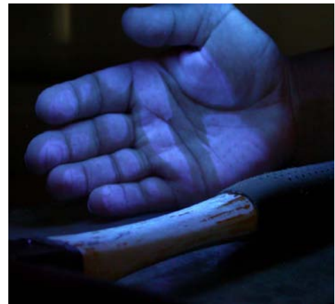
Figure 5: Hand (slightly creamed with moisturizer) after one-time touching a rubber coated hammer shaft. The spots where PAHs were transmitted due to contact with the rubber fluoresce in UV light. Holes in the coating become visible. Photograph: TÜV Rheinland Group
