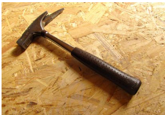
Figure 7: This hammer shaft is an example of a rubber-containing product Photograph: © Rainer-Sturm/ www.pixelio.de
